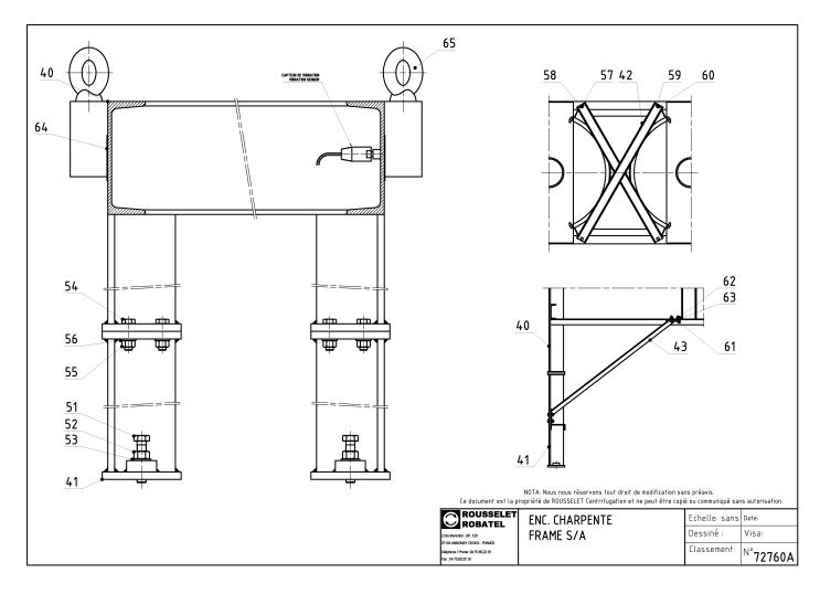
The support frame is equipped with legs and braces which are removed for shipment.
