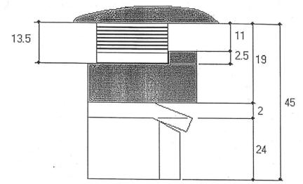
Figure 7. Spring compression height requirement.
