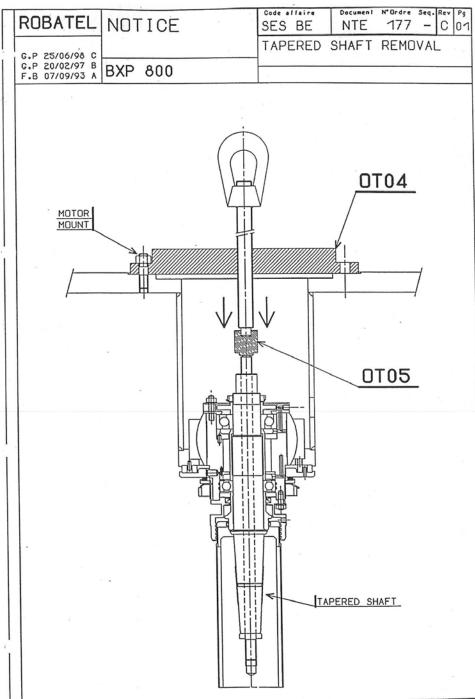
Figure 8. Page 1 of the disassembly / reassembly sketches.
