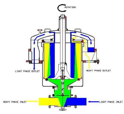
Figure 2. Single stage Rousselet Robatel BXP extraction flow diagram.
