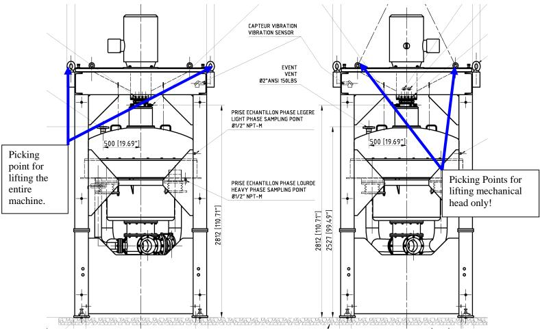
Figure 4. Extractor lifting points.
