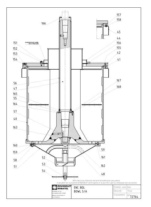
The bowl (ITEM NO. 40, DRAWING NO. 72764) has an internal diameter of 800 mm, a useful volume of 320 liters, and rotates at a speed of 1400 rpm at 70 Hz.
