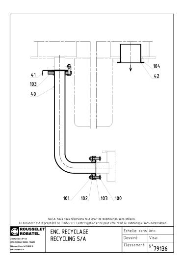
The casing of one stage is equipped with a recycling system for the heavy phase.
