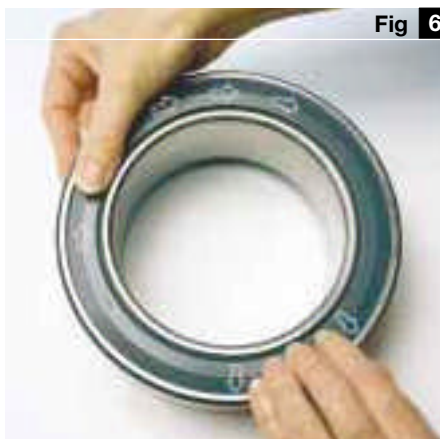
Inserting the seal in the outer ring
