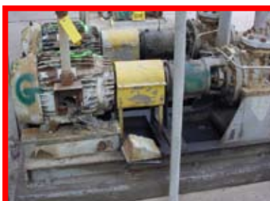
90776 Durco , Mark II, 40 GPM, 1.5" x 1" x 8", 200 ft head, Acero Inoxidable 316
