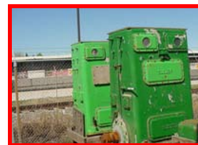
75505 Sulzer, 2D200-1D, 401 SCFM, 245 psi Suction pressure, 480 psi Discharge pressure
