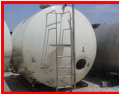
90644 5000 gal., 9' 0", 9' 6", ATMOS, CS OUTER/304SS INNER
