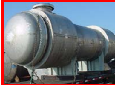
81273 Ohmstede, 12694 pies 2 , 304LSS/ 304LSS /304LSS, 305/302 psi, 300/300°F, Tipo BEM
