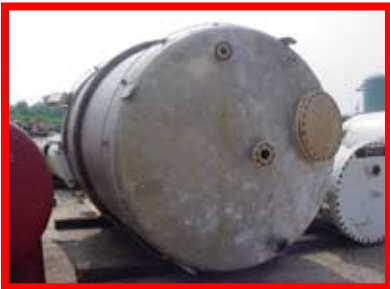
89298 Fabricated Products, 4800 gal., Acero Inoxidable, 8'6" x 11'4", 15 psi
