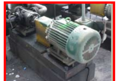
90782 IMO/Delaval, A324ATX-162, 101 GPM, 3x 2 1/2 29 HP
