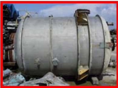
90612 Addison Fabricators, 4500 gal., 2205 DUPLEX SS, 8'0" x 9'9", 50 psi
