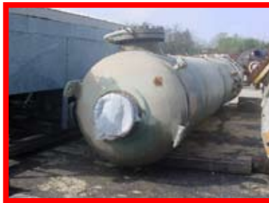
90731 Downington, 4300 gal., 316 SS CLAD, 5'0" x 28'0", 350 psi
