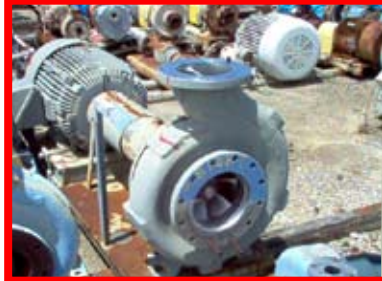
81087 Durco, MARK III, 1200 GPM, 10" x 8" x 16", 75 HP
