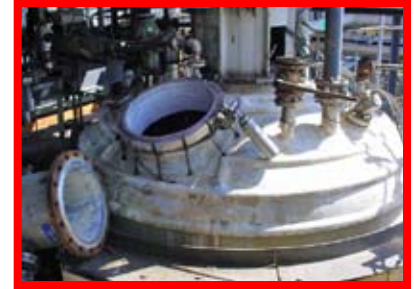
93651 3V-Cogeim, FPP-600-D-FV, 66.2 ft 2 , Nutsche, filtro/secador, Hastelloy C y Acero Inoxidable 316, 50 psi, Jacketed, 90 psi
