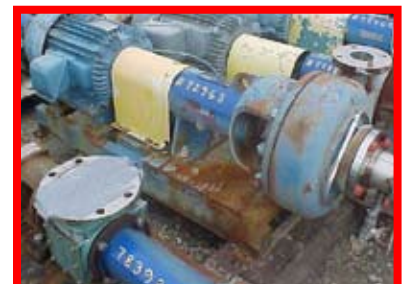
72963 Discflo, 403-2HHD, 175 GPM, 4" x 3" x 12', 15HP, 62 ft head
