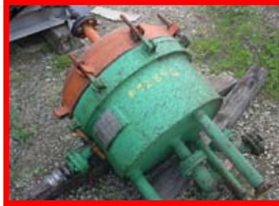
92846 SPARKLER, 33-S-7, Pressure Leaf, 13 pies 2 , Acero al Carbón
